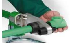
3.) Within the allowed time interval, connect the pipe and Fitting (do not twist)
