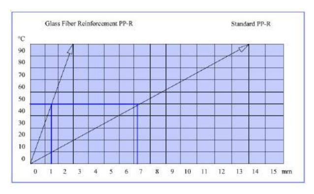
While fiberglass reinforced PP-Rc pipes elongate by 1.75mm per 1 meter at a temperature difference of 50°C, standard PP-Rc pipes elongate by 7.5mm per 1 meter under the same temperature difference.
